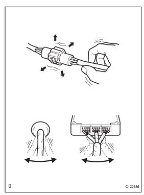
(d) While observing the screen, gently jiggle the connector or wire harness between the ECU and sensors, or between ECUs.
