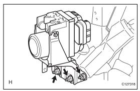
(b) Place tags or marks to identify the installation locations of each brake line.
