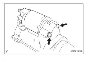
(d) Install the magnetic switch with the 2 screws. Torque: 7.5 N\*m (76 kgf\*cm, 66 in.\*lbf)
