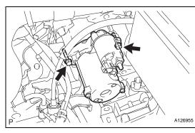
(c) Remove the 2 bolts and starter.
