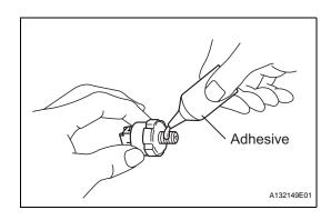
(h) Install the oil pressure switch.
