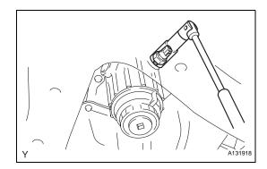
(b) Using a 24 mm deep socket wrench, remove the oil pressure switch.
