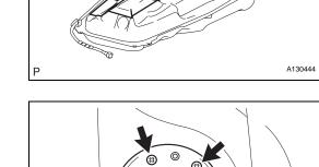
7. **REMOVE FUEL SENDER GAUGE ASSEMBLY** (a) Remove the 5 screws and sender gauge.
