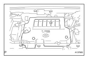
**79. INSTALL V-BANK COVER SUB-ASSEMBLY** (a) Attach the 3 clips to install the engine cover.
