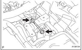
(g) Remove the bolt and nut, and disconnect the engine mounting insulator LH.
