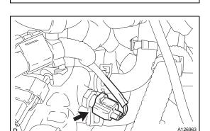
(c) Disconnect the engine coolant temperature sensor connector.
