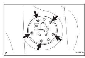
**REMOVE FUEL SENDER GAUGE ASSEMBLY** 7. (a) Remove the 5 screws and sender gauge.
