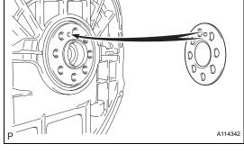
(e) Install the drive plate and rear spacer onto the crankshaft.
