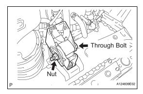
(b) Install the through bolt and nut which is used to secure the front engine mounting bracket FR. HINT:
