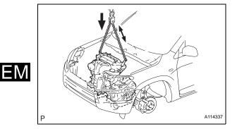
(b) Lower the engine out of the vehicle slowly and carefully.
