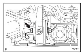
(b) Install the through bolt which is used to secure the rear engine mounting insulator, into the rear engine mounting bracket.
