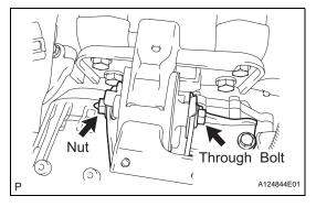
(b) Install the engine mounting insulator LH with the through bolt and nut.
