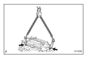
(b) Attach the sling device and the engine with the chain block.
