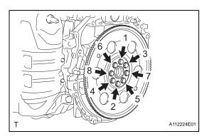
(f) Using several steps, uniformly install and tighten the 8 bolts in the sequence shown in the illustration.
