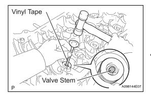
(d) Using a plastic-faced hammer and discarded valve (with its tip wrapped with tape), lightly tap the installed valve to fit it into place.
