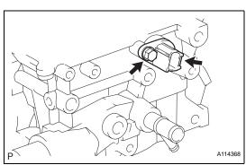
(b) Align the bearing claw with the claw groove of No. 1 and No. 2 bearing cap, and push in the No. 1 camshaft bearing.
