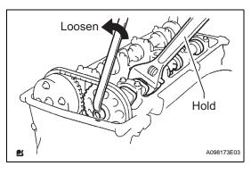
(c) While holding the camshaft with a wrench, loosen the camshaft timing set bolt.
