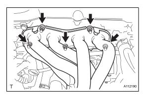
(b) Remove the 5 nuts, manifold converter and gasket.
