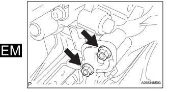
(b) Remove the 2 nuts, tensioner and gasket.
