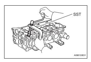
(b) Using SST, compress the spring, then remove the 2 retainer locks.
