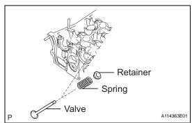
(c) Remove the retainer, spring and valve from the cylinder head.
