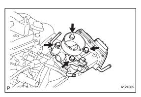
(b) Install the throttle body and fuel pipe clamp with the 4 bolts.
