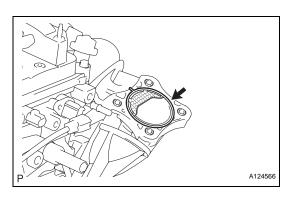
Remove the gasket from the intake manifold.
