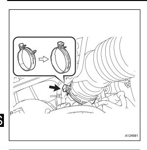
(f) Lock the No. 1 air cleaner hose clamp, and then disconnect the No. 1 air cleaner hose from the throttle body.
