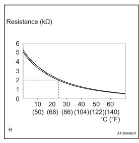
The battery temperature sensor installed on the battery current sensor detects battery temperature.
