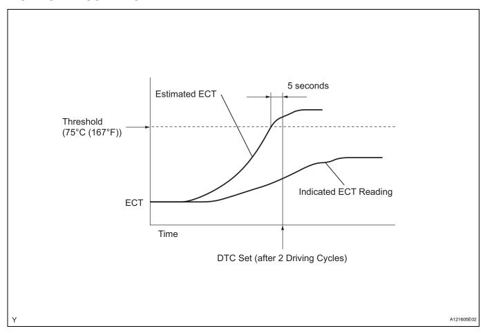
The ECM estimates the ECT based on the starting temperature, engine loads, and engine speeds. The ECM then compares the estimated temperature with the actual ECT. When the estimated ECT reaches 75°C (167°F), the ECM checks the actual ECT. If the actual ECT is less than 75°C (167°F), the ECM interprets this as a malfunction in the thermostat or the engine cooling system and sets the DTC.
