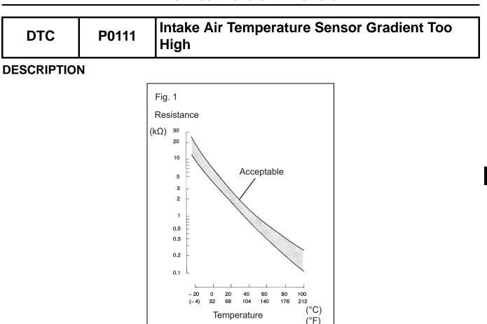
The Intake Air Temperature (IAT) sensor, mounted on the Mass Air Flow (MAF) meter, monitors the IAT. The IAT sensor has a built-in thermistor with a resistance that varies according to the temperature of the intake air. When the IAT is low, the resistance of the thermistor increases. When the temperature is high, the resistance drops. These variations in resistance are transmitted to the ECM as voltage changes (See Fig. 1).
