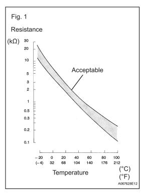
The Intake Air Temperature (IAT) sensor, mounted on the Mass Air Flow (MAF) meter, monitors the IAT. The IAT sensor has a built-in thermistor with a resistance that varies according to the temperature of the intake air. When the IAT is low, the resistance of the thermistor increases. When the temperature is high, the resistance drops. These variations in resistance are transmitted to the ECM as voltage changes (see Fig. 1).
