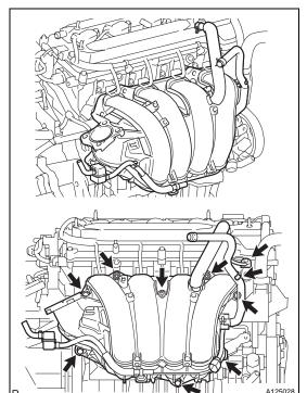
(b) Install the intake manifold with the 5 bolts and 2 nuts.
