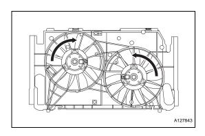
(c) Check that the cooling fan rotates.
