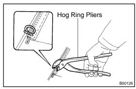
Using hog ring pliers, install the cushion cover to the cush-(a) ion pad with new hog rings.
