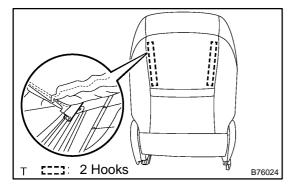
(e) Using a screwdriver, disengage the 2 hooks and remove the seatback cover together with the pad.
