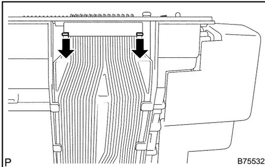
**11. REMOVE METER CIRCUIT PLATE NO.3****NOTICE:**
