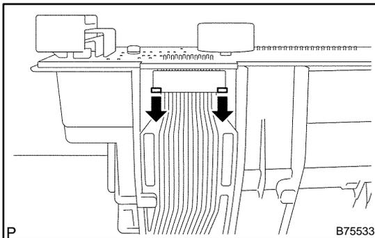
**12. REMOVE METER CIRCUIT PLATE NO.4****NOTICE:**
