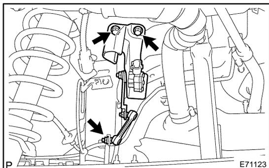
1. **REMOVE HEIGHT CONTROL SENSOR SUB-ASSY REAR**
