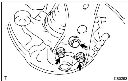
**40. INSTALL FRONT SUSPENSION ARM SUB-ASSY LOWER NO.1 LH**
