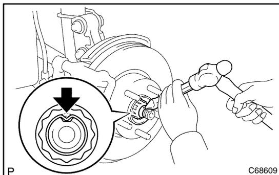
**43. INSTALL FRONT AXLE HUB LH NUT**
