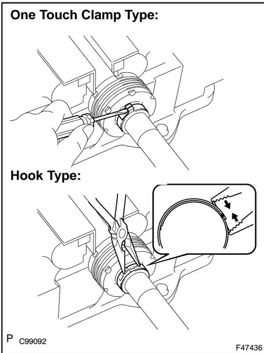
**16. REMOVE DRIVE SHAFT DAMPER SETTING CLAMP**
