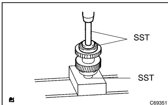
(b) Using SST and a press, install a new bearing into the counter drive gear.
