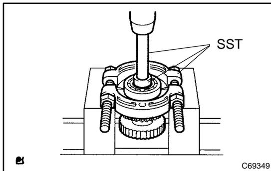
(b) Using SST and a press, remove the bearing from the counter drive gear.
