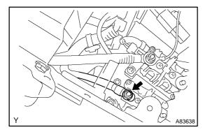
(c) Install the main battery cable with a new nut.
