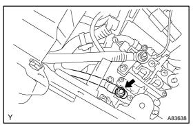
(b) Remove the nut, then disconnect the main battery cable.
