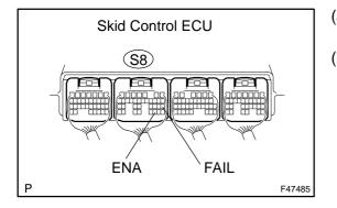
(a) Check the waveform between terminal S8–20 (FAIL) and the ground of the skid control ECU using an oscilloscope.
