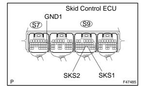
(a) Measure the voltage according to the value(s) in the table below.
