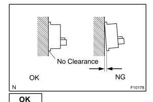
(a) Check the sensor installation.
