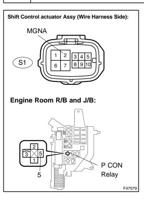
(a) Measure the resistance according to the value(s) in the table below.
