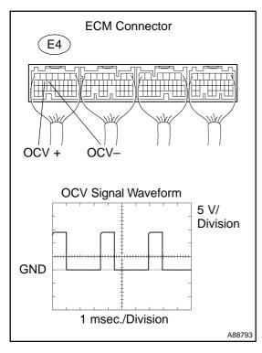
(a) During idling, check the waveform between the specified terminals of the E4 ECM connector using an oscilloscope. **Standard:**
