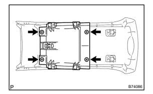
(1) Remove the 4 screws and then the rear console box cup holder.
