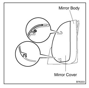
(b) After installing the outer mirror cover, check that there is no gap between the cover and mirror body.
