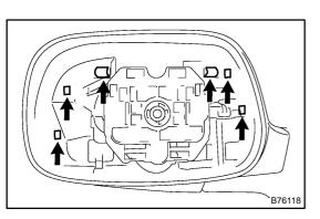
(b) Disengage the 6 claws and remove the mirror cover.
