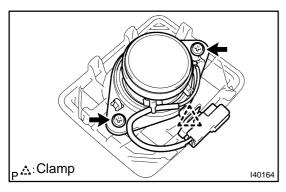
(c) Remove the 2 screws and disengage the clamp and then remove the stereo component speaker assy front.
