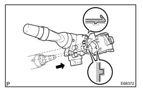
(c) Disengage the claws and remove the headlamp dimmer switch assy.
