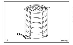
Front Seat Airbag Assy LH Battery SST 10 m (33ft) or more (3) Tie the tires together with 2 wire harnesses.
