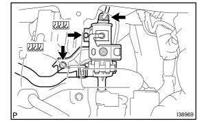
(b) Install the heater water pump assy with the 2 bolts. **NOTICE:**
