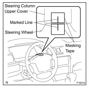
(3) Draw a line on the masking tape as shown in the illustration.
