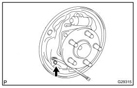
(c) Connect the parking brake cable assy No.3 to the backing plate with a bolt.
