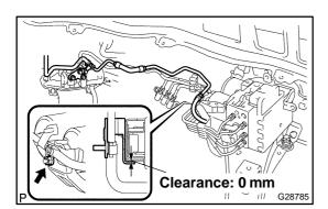
(e) Set the brake actuator tube assy with the nut. Torque: 8.5 N·m (87 kgf·cm, 75 in. lbf)
