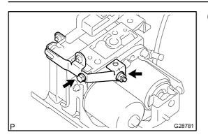
(b) Remove the bolt, nut, and the bracket from the brake actuator assy.
