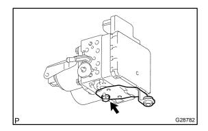
(d) Remove the bolt and brake actuator bracket No.2 from the brake actuator assy.
