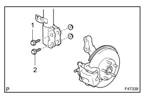
Check installed bolts combination. Select appropriate bolts from the table below to adjust the camber to within the specified range.
