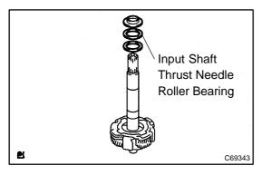
(b) Remove the input shaft thrust bearing race No.1, No.2 and input shaft thrust needle roller No.1 bearing.
