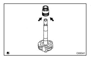
6. INSTALL PLANETARY SUN GEAR SUB-ASSY
