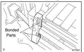
31. INSTALL BATTERY CLAMP PAD (BATTERY CARRIER CUSHION NO.1)
