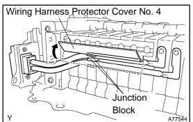
(c) Flip open the wiring harness protector cover No. 4 shown in the illustration, then remove the service plug from the junction block.
