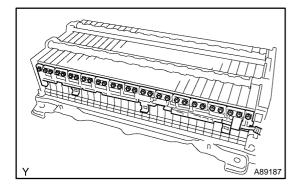
(c) Remove the 26 nuts and frame wire No. 2.
