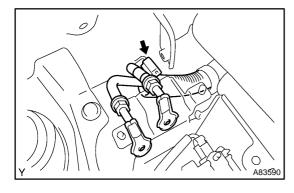
(c) Install the frame wire to the rear floor panel with the clamp.
