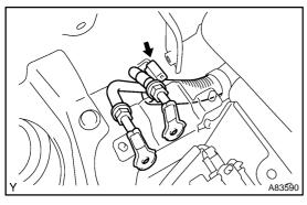
(b) Remove the clamps, then remove the frame wire from the rear floor.
