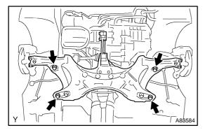
(b) Remove the 4 bolts shown in the illustration from the front suspension crossmember.
