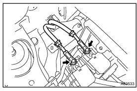
(d) Install the frame wire to the system main relay No. 2 and No. 3 with 2 new nuts.
