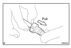
(2) After connecting the fuel tube connector, check that the fuel tube connector and pipe are securely connected by pulling them.
