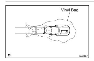
(5) Cover the disconnected fuel tube connector and pipe with a vinyl bag to prevent damage and intrusion of foreign objects.
