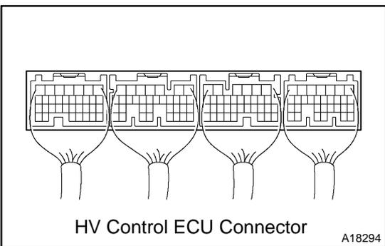
(a) Check the connection condition of all the connectors at the HV control ECU.
