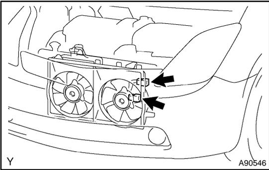
(a) Check the connection condition of the cooling fan motor connectors.
