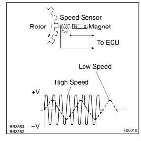
The speed sensor detects wheel speed and sends the appropriate signals to the ECU. These signals are used to control the ABS control system. The front and rear rotors have 48 serrations, respectively.
