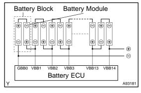
The HV battery assembly consists of nickel hydride batteries. Nickel hydride batteries do not require external charging. The SOC (state of charge) of the HV battery is maintained at a constant voltage level by the HV control ECU while the vehicle is being driven. In the HV battery assembly, 28 modules are connected in series, and each module has six 1.2 V cells that are connected in series. Thus, the HV battery assembly contains a total of 168 cells which produce 201.6 V.
